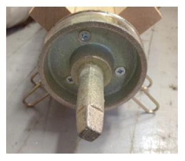
Affix the friction brake drum to the right side of the loom using 3x screws no 14, 2"
