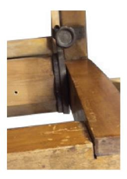
Take the warp beam out of the loom and remove all the metal pieces on both side of the back beam. Remove also the ratchet, rod and brake treadle from the loom.
